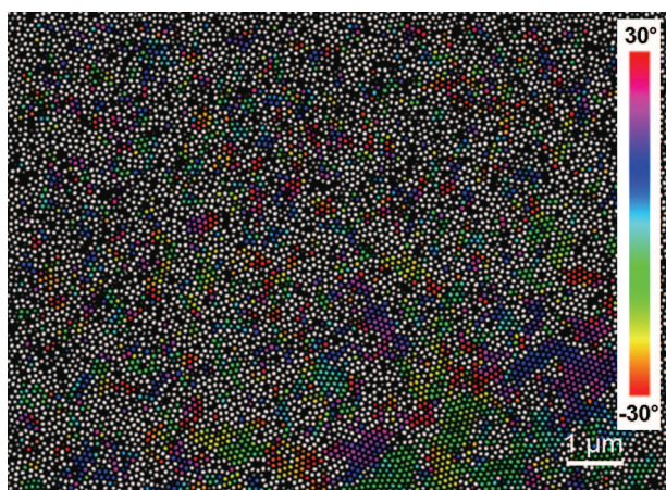
Figure 9. SEM image of porous alumina ( U = 65 V, 0.03 M H_2SO_4 , t = 15 min, hard anodization) containing 9006 pores. The pores are color-coded on the basis of the average of the (6 NN) angles of the considered pore.
