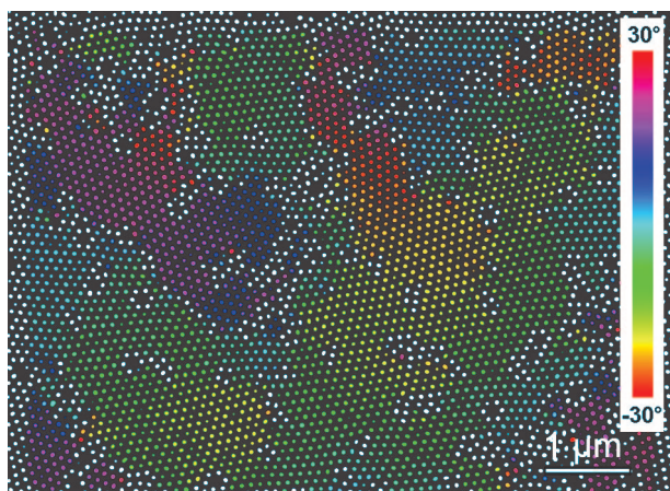
Figure 7. SEM image of porous alumina ( U = 65 V, 0.03 M \text{H}_2\text{SO}_4 , t = 60 min, hard anodization) containing 4393 pores. The pores are color-coded on the basis of the average of the (6 NN) angles of the considered pore.
